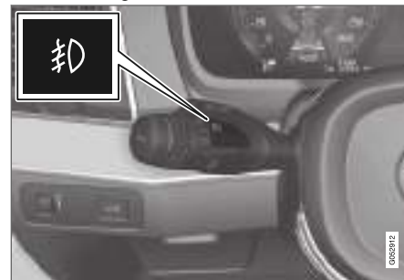
Button for front fog lamps.
