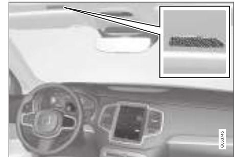
Voice control system microphone
