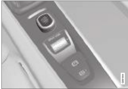
Start knob in the tunnel console.
