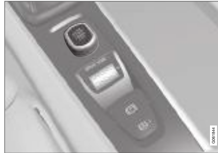
Start knob in the tunnel console.
