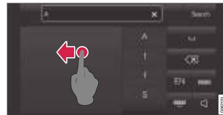
Delete all characters in the text field (2) by swiping across the handwriting field (1).
