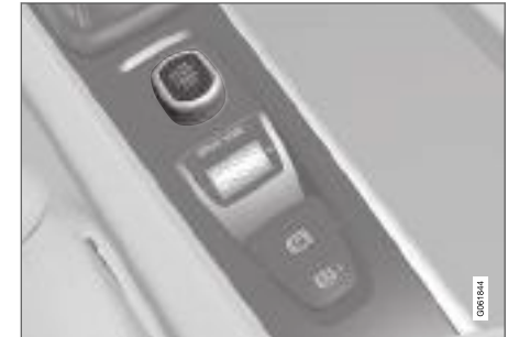
Start knob in the tunnel console.
