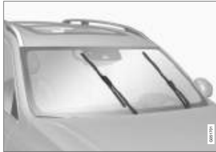
Wiper blades in service position.
