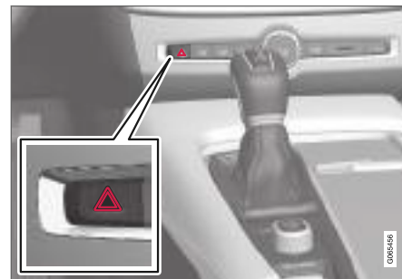
Button for hazard warning flashers.
