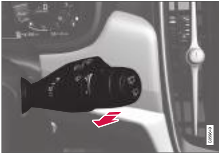
Washing function, right-hand stalk switch.
