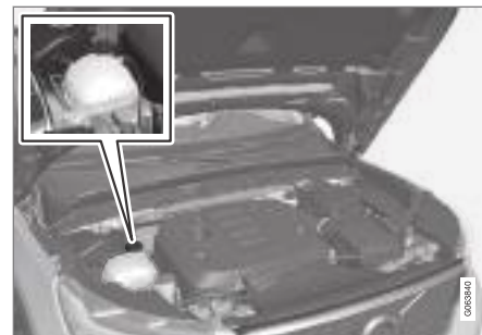
Coolant expansion tank.
