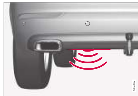
The sensor is located on left of centre in the bumper.
