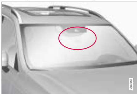
Location of the camera unit.
