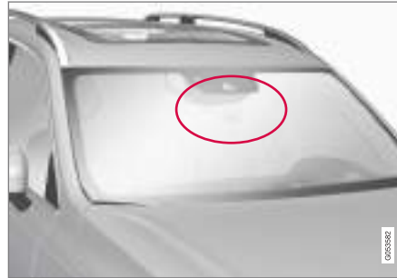
Radar unit location.
