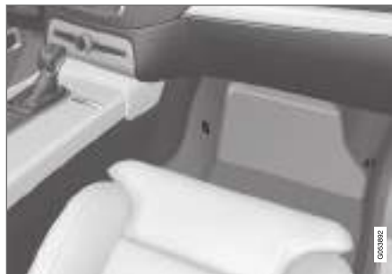
Mounting point locations in the front seat.
