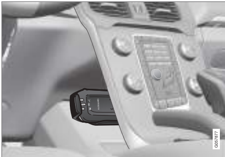
Handheld unit storage location.
