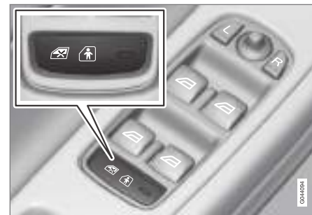
Control panel driver's door.
