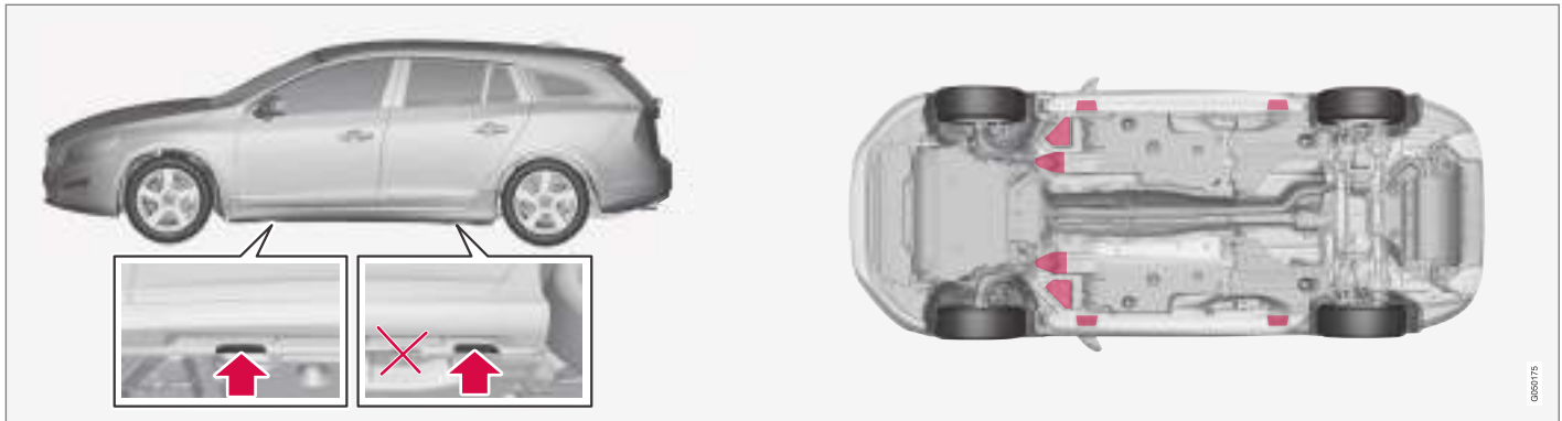
Jacking points (arrows) for the jack that belongs to the car and lifting points (marked in red).
