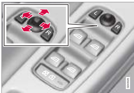
Controls for door mirrors.
