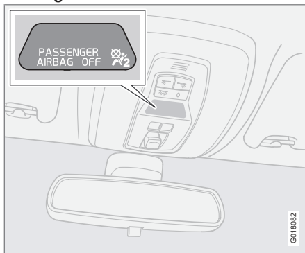
Indicator showing that the passenger airbag is deactivated.
