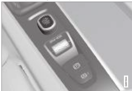
Start knob in the tunnel console.
