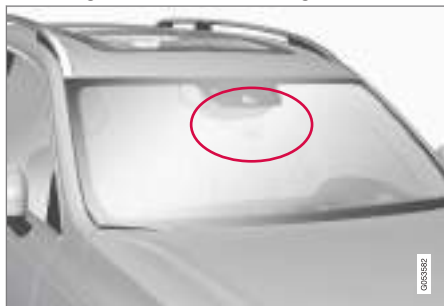
Location of the camera unit
