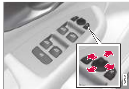
Controls for door mirrors.
