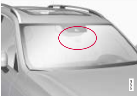
Radar unit location
