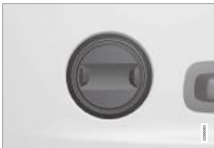
Control in cars with two-way lumbar support*.
