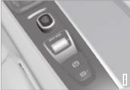
Start knob in the tunnel console.
