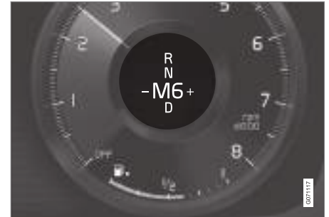
Overview of the shift pattern in the driver display for small gear lever.
