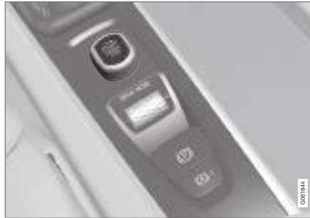
Start knob in the tunnel console.
