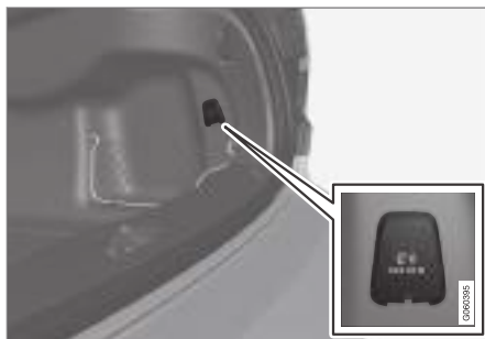
12 V electrical socket in cargo area*.
