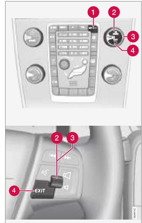
Control panel in centre console and steering wheel keypad. The figure is schematic - the number of functions and layout of the buttons both
