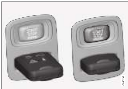
Ignition switch with remote control key extracted/inserted.
