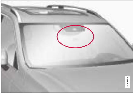
Radar unit location.
