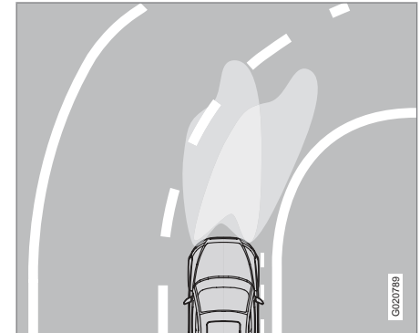
Headlamp pattern with function deactivated (left) and activated (right) respectively.
