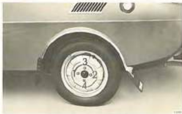
Order of tightening wheel nuts
