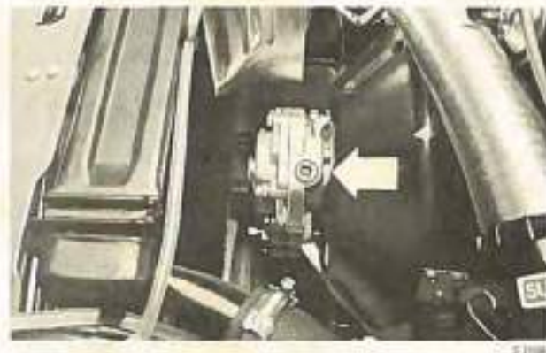
Filler plug, manual transmission, version 1
