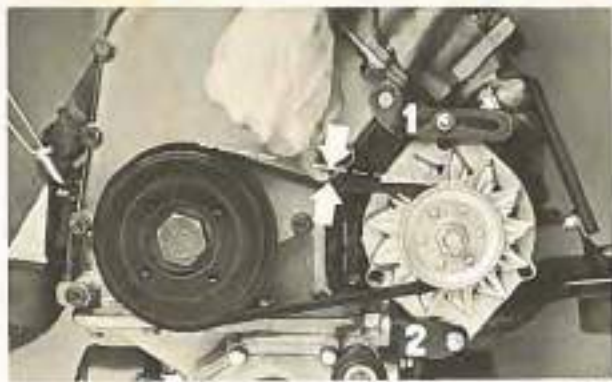
Alternator belt tension
