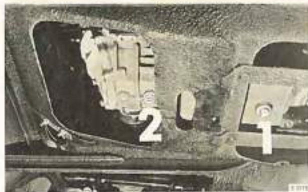
Drain plugs, manual transmission
