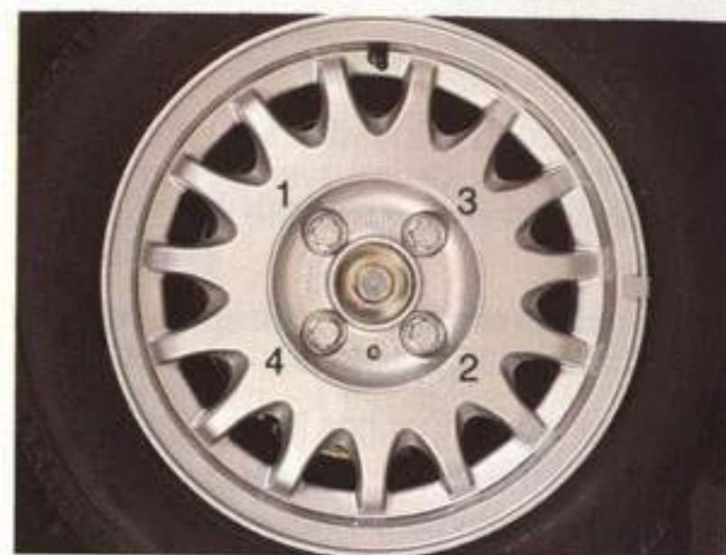
Tightening sequence for wheel studs
