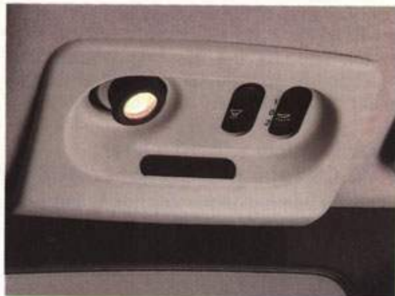
Switch for interior lighting
