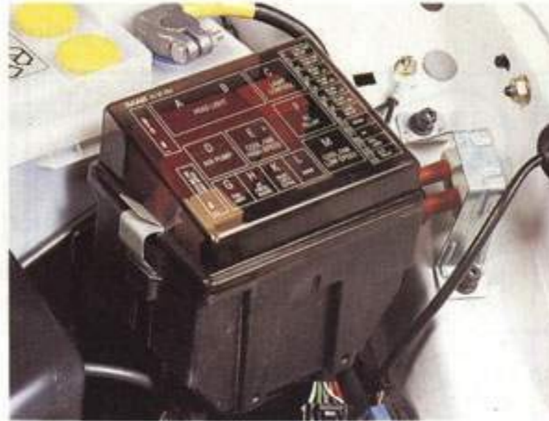
Power distribution panel in engine compartment SG1301
