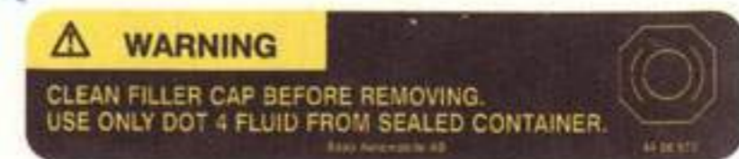
Brake system: Clean filler cap before removing. Use only DOT 4 fluid from sealed container.
