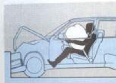
The airbag is completely inflated.
