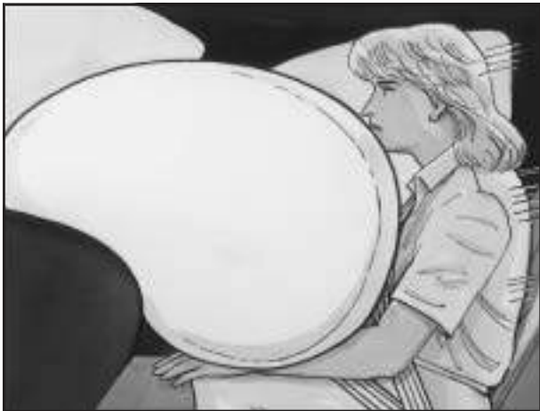
The right front passenger's airbag is in the instrument panel on the passenger's side.
