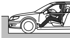
Sensor detects deceleration and sends a signal via the control module to a gas generator that inflates the airbag.
