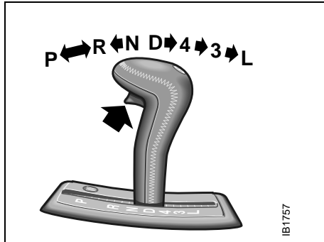
Detent positions for selector movement
