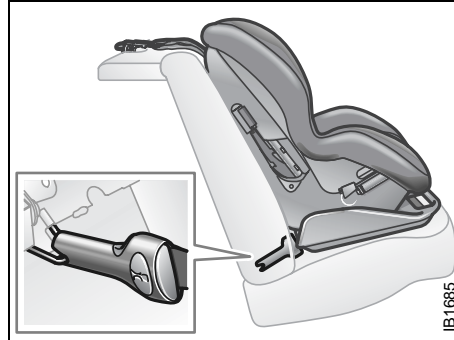
Semi-rigid 2-point lower attachment with top tether
