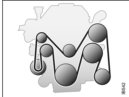
Routing of the Poly-V-belt: 4-cylinder engine
