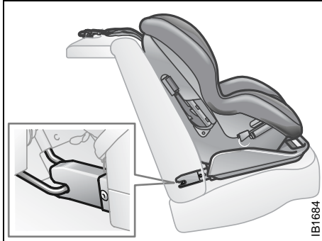
Rigid 2-point lower attachment with top tether
