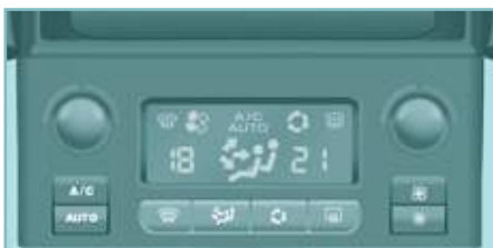
Digital controls, with separate driver and passenger settings
