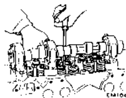
Fig. 38 Removing rocker arm
