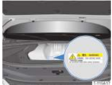
High-voltage Components Warning Labels
