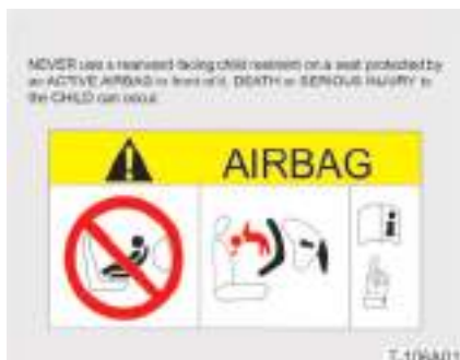
Warning label on front passenger sun visor
