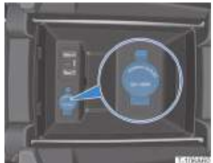
12V on-board power supply in centre console cubby
