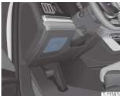
Dashboard fuse box
