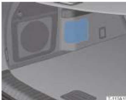
Rear compartment fuse box
