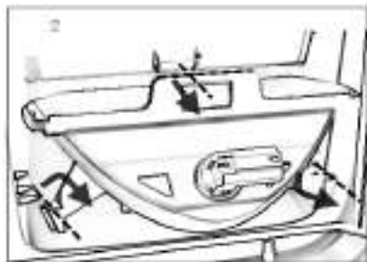
2. Remove high mount brake light assembly.
