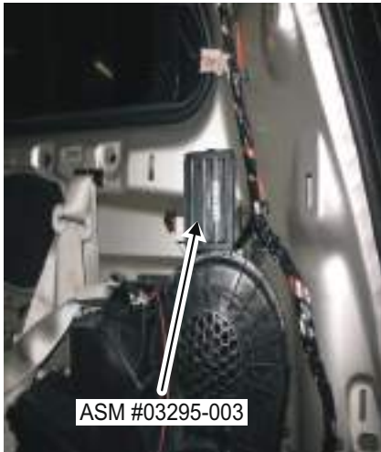
OTC Remote Receiver (Behind Rear Passenger Quarter Panel Above Rear Heat Unit)
