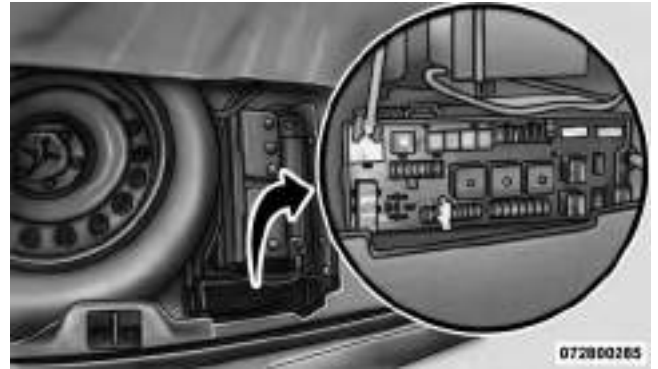
Rear Power Distribution Center
