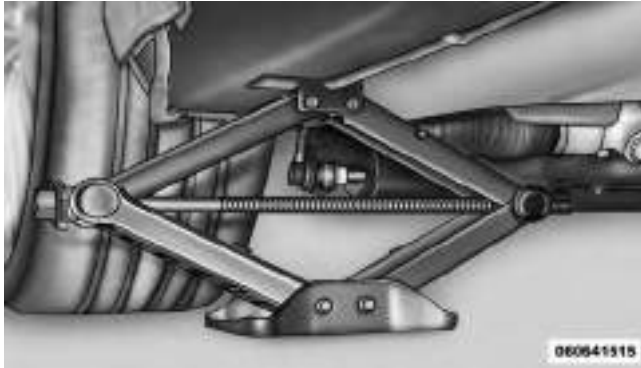
Front Jacking Location
