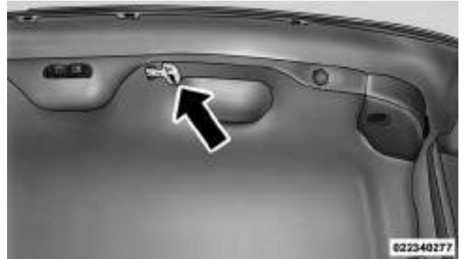
Trunk Emergency Internal Release
