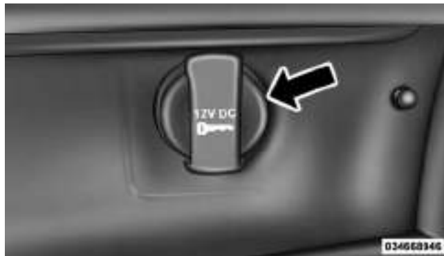
Front Power Outlet
