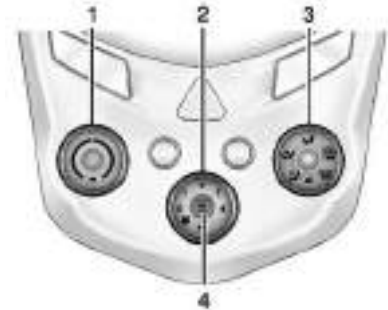
Climate Control System with Heater Only
