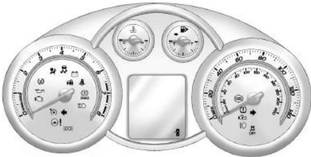
English Gas Cluster with Automatic Transmission Shown, Metric and Manual Transmission Similar
