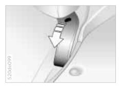
The strap for the belt guide can be opened: release the push button.
