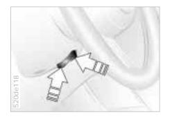
Press button: set the steering wheel vertical to the seating position.
