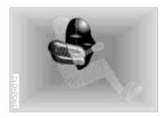
Deceleration sensors continuously monitor the acceleration forces acting upon the vehicle. If, as the result of a frontal collision, a deceleration is reached at which the protection of the safety belts alone is no longer adequate, the gas generators of the driver and passenger airbags are ignited. However, the passenger airbag is only triggered if an additional sensor has recognized that the passenger seat is occupied.
