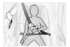
The illustration shows the correct seating position for an older child wearing a safety belt with sufficient distance between him and the side airbag (arrow).
