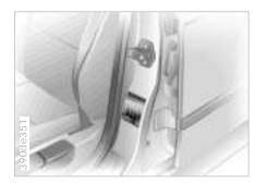
The inflation pressures are indicated on a label attached to the B-pillar behind the driver's door (visible with door open).
