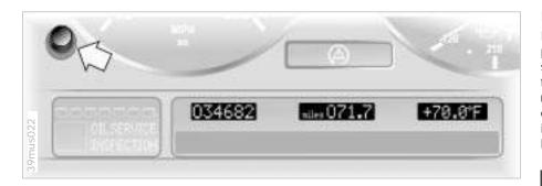
Odometer, outside temperature display
