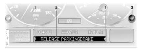
Text messages are used to alert the driver to system malfunctions with the ignition key in position 2 and higher. The alert is accompanied by a gong.
