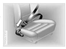
The safety belt tensioner responds to severe frontal collisions by tightening the belts to ensure that occupants remain firmly positioned in their seats. A gas-pressure system retracts the buckle assembly to tension the shoulder and lap belts within fractions of a second. This reduces the tendency to slide under the lap belt.
