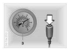
8 Press and hold the button for operating the compressor. Watch the pressure gauge carefully as you do so. As long as the pressure reading is between approx. 5–8 bar, sealant is being forced into the tire. When the pressure gauge falls significantly below approx. 5–8 bar while the compressor is operating, all of the sealant is in the tire. Air is being pumped into the tire.
