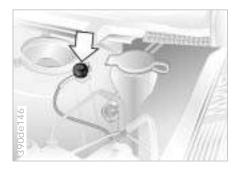
5 Then connect the negative terminals. Attach the cable to either the support vehicle's negative battery terminal (-), or to a suitable ground on its engine or bodywork. Then connect the other end of the cable to a ground on the engine or on the bodywork of the vehicle that is to be started. There is a special nut on the strut dome of your BMW for this (refer to the arrow in the illustration).
