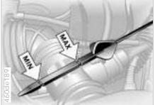
The oil volume between the two marks on the dipstick corresponds to approx. 1.1 US quarts (1 liter). Do not fill beyond the upper mark on the dipstick. Excess oil will damage the engine.
