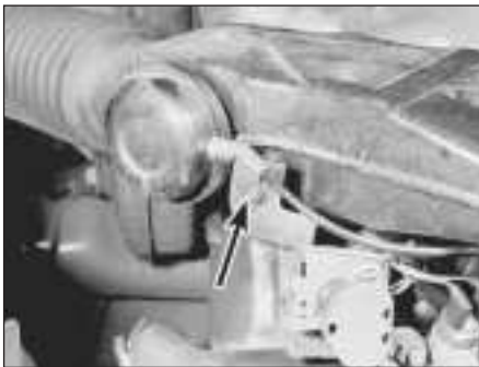
8.7 Air cleaner mounting bracket nut (arrowed)
