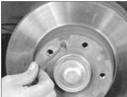
5.6a Remove the disc retaining screw . . .
