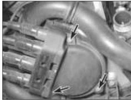
8.18 Remove the three bolts (arrowed) from the distributor cap
