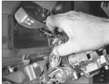
6.2 Squeeze the tabs to release the switch from the mounting
