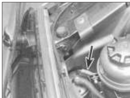
33.2 Inspect the hoses (arrowed) at the top of the evaporative emissions charcoal canister for damage
