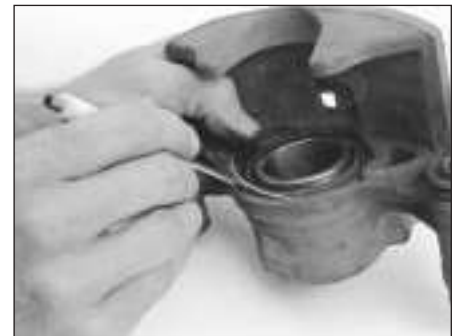
4.4b Remove the circlip for the dust seal
