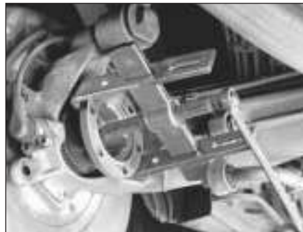
15.11 Remove the drive flange with a puller
