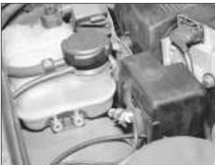
4.9b On other models, the expansion tank (coolant reservoir) is located on the side of the engine compartment - remove the cap to add coolant
