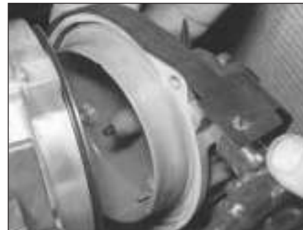
9.6a Unbolt the distributor cap (M40 engine) . . .
