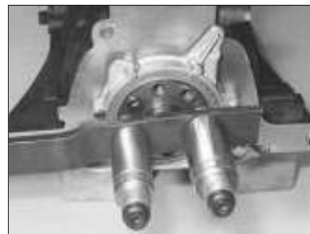
10.12a Home-made tool for holding the crankshaft stationary while the crankshaft pulley bolt is being loosened (engine removed for clarity)
