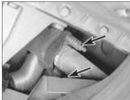
6.5a Remove the exhaust manifold nuts (arrowed) from the exhaust pipe (M20 engine) - soaking the nuts with penetrating oil should make them easier to remove
