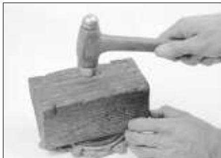
16.7 Drive the new seal into the retainer with a block of wood, or a section of pipe, if you have one large enough - make sure the seal enters the retainer bore squarely
