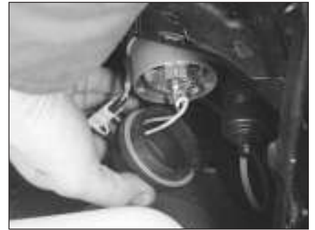
12.9 Twist and release the headlight inner cover
