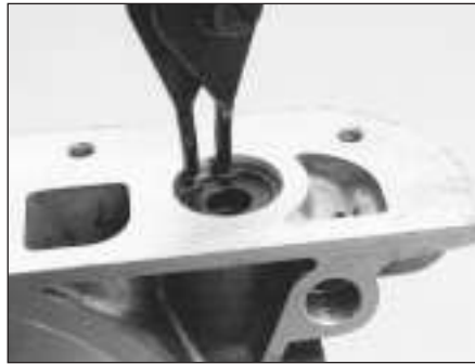
14.27a Extract the circlip from the oil pump (M40 engine) . . .
