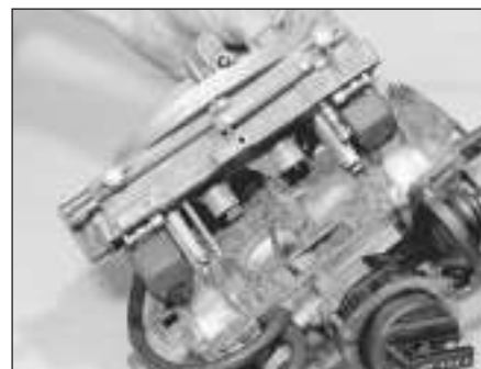
12.6a Lifting the cover from the carburettor main body
