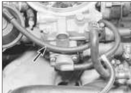
11.6 Note the locations of the carburettor vacuum hoses (arrowed) before disconnecting them
