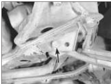
4.6a If you're removing the control arm, remove the self-locking nut and the through-bolt (arrowed) that attach the inner end of the arm to the vehicle
