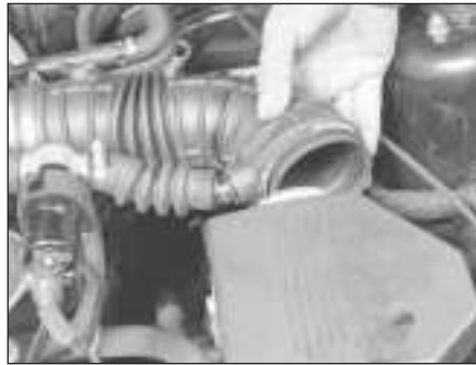
20.4 Detach the duct from the air cleaner housing
