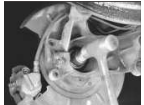
15.12 Using a soft-faced hammer, drive the stub axle out of the bearing
