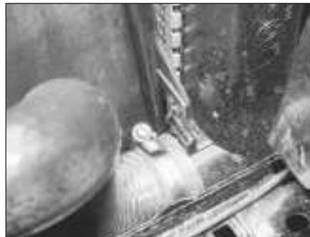
4.3b Bottom hose connection to the radiator
