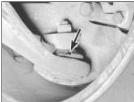
24.10 Inspect the balljoint boots for tears (arrowed)
