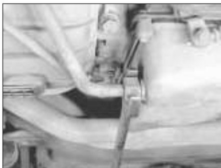
28.5a Unscrew the dipstick tube collar
