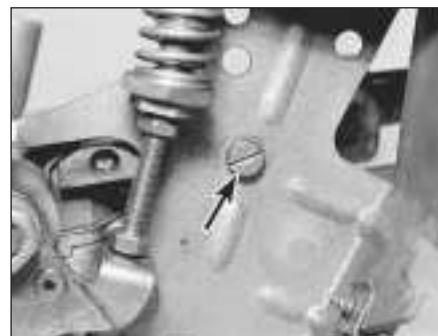
12.7 Throttle positioner bracket-to-throttle housing screw (arrowed)
