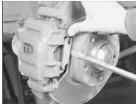
3.5h Prise off the anti-rattle spring (5-Series)
