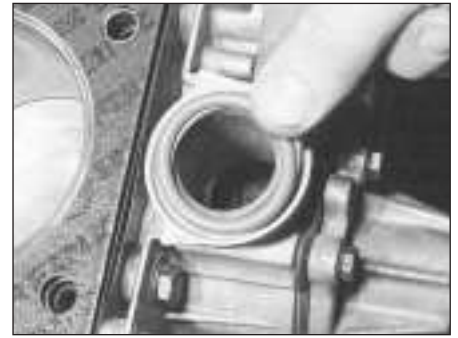
12.26 Fitting a new rubber O-ring in the groove in the top of the oil pump/front end cover on the M40 engine
