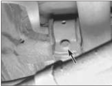
12.2 Rear anti-roll bar bracket bolt (arrowed) (3-Series)
