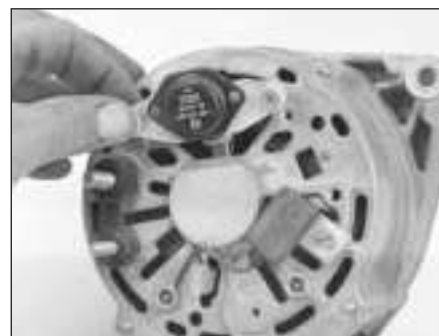
16.4b The regulator can be withdrawn easily on Bosch alternators. This type of regulator is integral with the brush assembly
