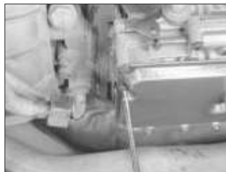
28.10a Use a Torx key to remove the filter bolts . . .
