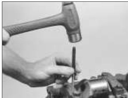
13.4 Use a centre-punch or number-stamping dies to mark the main bearing caps to ensure refitting in their original locations on the block (make the punch marks near one of the bolt heads)
