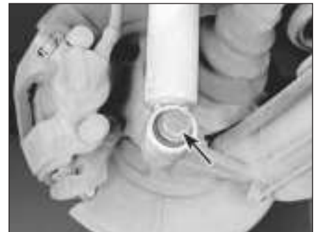
9.3 Remove the shock absorber lower mounting bolt (arrowed)
