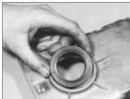
11.7 The crankshaft front oil seal is pressed into the front of the lower timing chain cover (cover removed from the engine for clarity)
