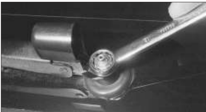
16.9 Removing the tailgate wiper arm nut (3-Series)
