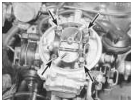
11.9 Unscrew the four bolts (arrowed) and lift the carburettor from the intake manifold
