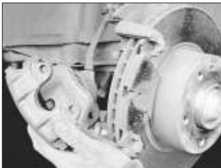
3.5j Remove the caliper and inner brake pad (5-Series)
