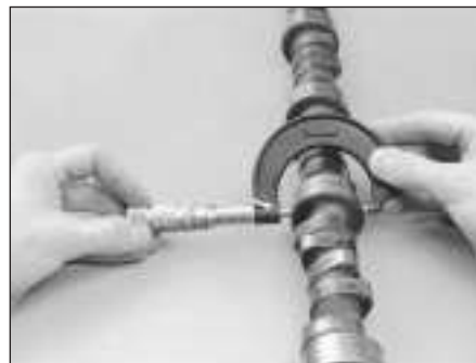
9.25 Measure each camshaft bearing journal and its corresponding bearing diameter in the cylinder head, then subtract the journal diameter from the bearing inside diameter to obtain the oil clearance
