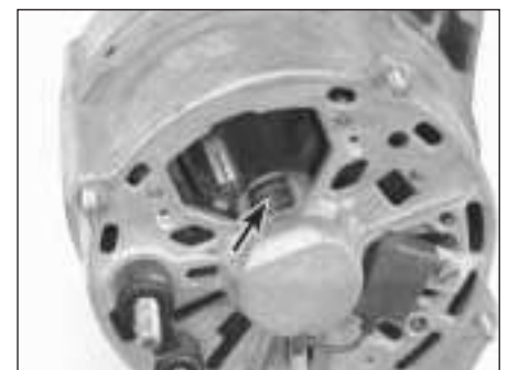
16.5 Use a torch to check the slip rings for scoring or deep grooves
