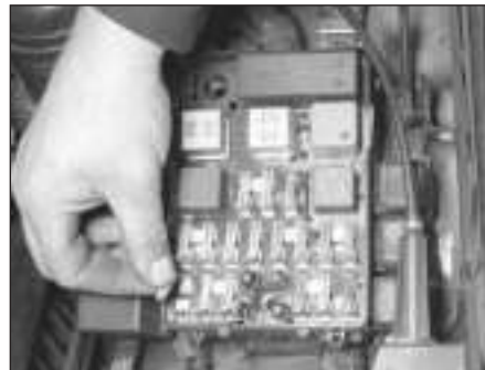
2.1b Removing the fuel pump fuse on 5-Series models
