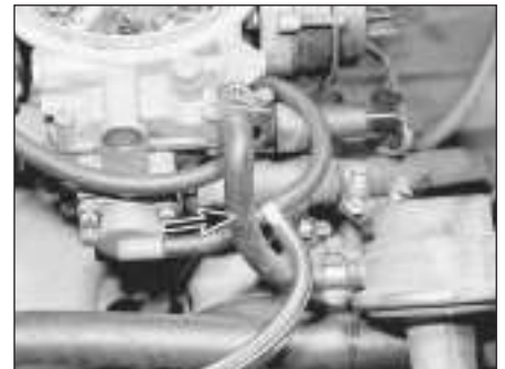
11.8 Disconnect the fuel supply hose (arrowed)
