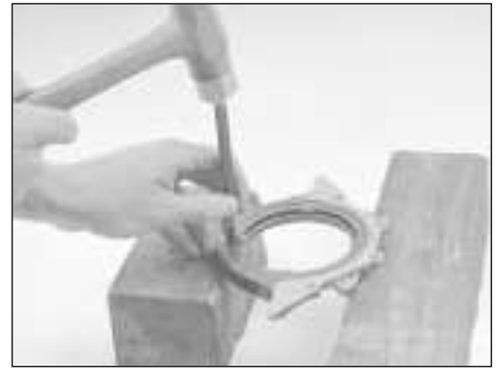
16.6 After removing the retainer from the block, support it on two wood blocks, and drive out the old seal with a punch and hammer
