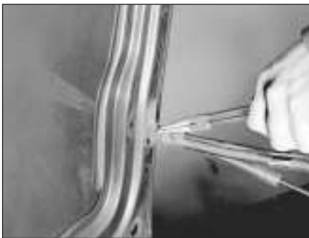
10.9 Pull off the clip with needle-nose pliers
