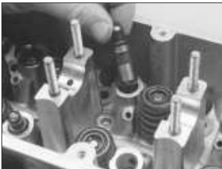
8.20c . . . then lift out the hydraulic tappets
