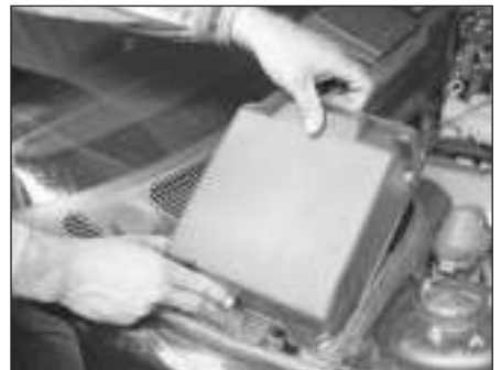
3.6c On all 1989 and later models, remove the four bolts and the protective cover to gain access to the fuel pump relay and ECU . . .
