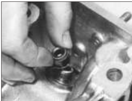
11.4a Lubricate the valve guide seal, and place it on the guide (the valve should be in place too) . . .
