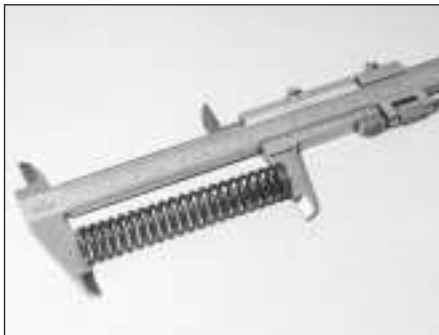
14.27e Checking the length of the pressure relief valve spring (M40 engine)
