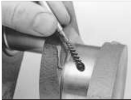
19.2 Use a wire or stiff plastic bristle brush to clean the oil passages in the crankshaft
