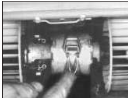
9.5b . . . and unclip the centre strap that secures the blower motor assembly
