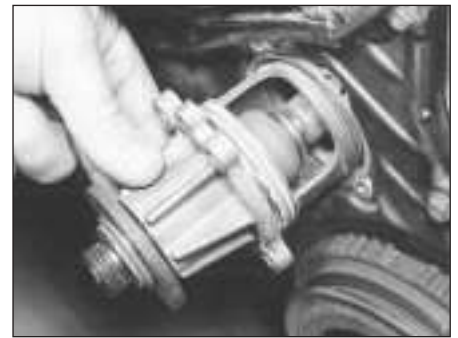
7.18b . . . and remove the water pump (M40 engine)
