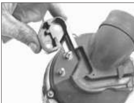
16.4a Remove the nuts and lift off the small terminal protector from the alternator cover, then remove the nuts and the cover
