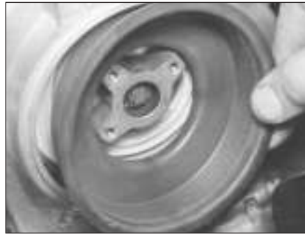
9.6c ... and remove the black plastic cover
