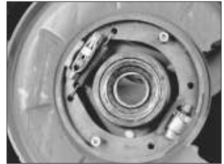
12.9 When you're done, the actuator should be properly seated between the two shoes as shown (hub removed for clarity)
