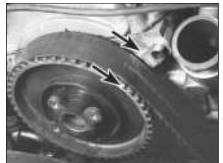
10.5b Align the mark on the camshaft sprocket with the mark on the cylinder head (arrowed)
