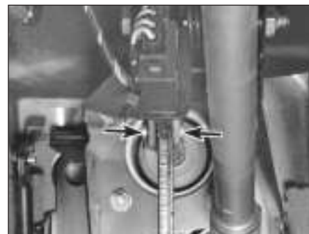
8.9 Disconnect the brake pedal return spring, then remove the clip and clevis pin (arrows) to disconnect the pushrod from the brake pedal (left-hand-drive models)
