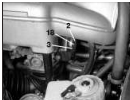
4.28a The TPS on L-Jetronic systems is located under the intake manifold (terminals arrowed)
