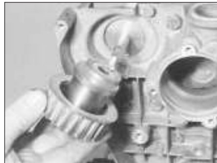
14.8 Removing the timing belt tensioner (M40 engine)
