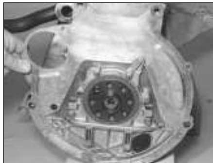
5.26 Removing the engine rear plate - M40 engine
