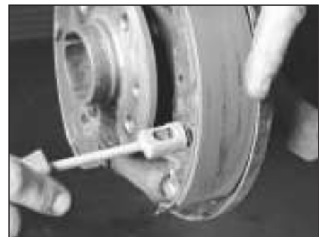
6.6b . . . and the rear shoe hold-down spring
