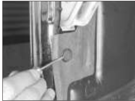
10.8a Use a small screwdriver to prise out the clip pin, then . . .
