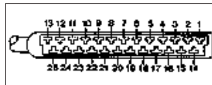
16.5 The ECU is located under the right-hand side of the facia. Unplug the electrical connector, and check the resistance between terminals 7 and 8 as in paragraph 3. The test results should be the same.
