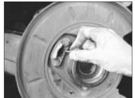
10.6 Pull the cable out of its conduit; before you refit the new cable, be sure to lubricate it with multi-purpose grease
