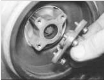
9.6b ... then unbolt the rotor ...
