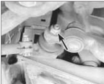
20.4 To remove an outer track rod, remove this nut (arrowed) from the end of the centre track rod, and use a balljoint separator to separate the balljoint stud from the centre track rod (if you're renewing the inner track rod end, mark the threads with paint before loosening the clamp bolt and nut)
