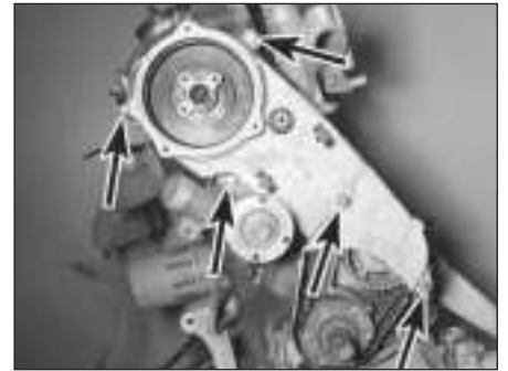
9.8 Remove all the nuts/ bolts (arrowed) that attach the upper and lower covers (M20 engine - removed for clarity)
