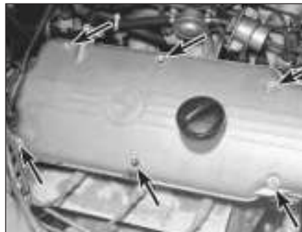
4.6a Valve cover bolt locations (arrowed) on M10 four-cylinder engines
