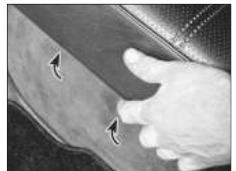
20.3 Grasp the seat at the front edge and pull up sharply (Saloon/Convertible models)
