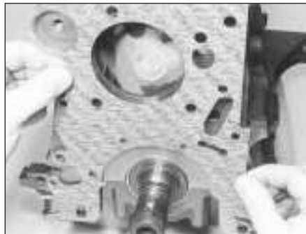
14.30 Locating a new gasket on the front of the cylinder block (M40 engine)
