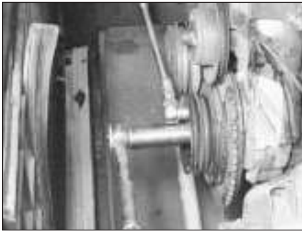
7.7 Place a socket and ratchet on the centre bolt to keep the pulley stationary, and use another socket and ratchet to remove the smaller bolts attaching the pulley to the vibration damper
