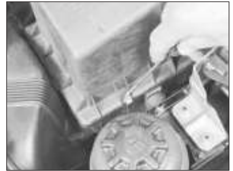
20.5 Use a screwdriver to detach the air cleaner cover clips
