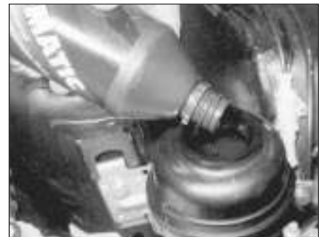
7.6 Adding fluid to the power steering reservoir
