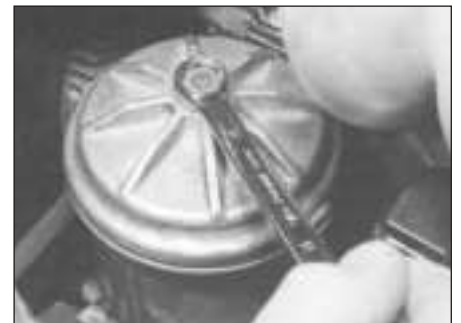
6.17a Unscrew the bolt . . .
