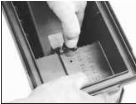
16.11a Push the tab and remove the air duct from inside the air cleaner assembly
