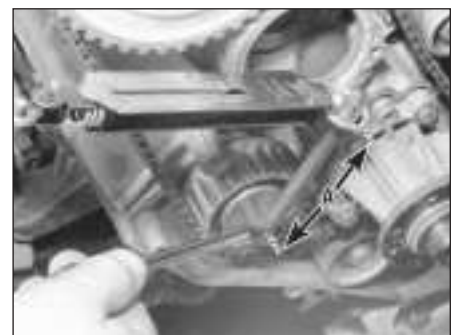
10.23b Using a spring balance and Allen key to adjust the tension of the timing belt on the M40 engine
