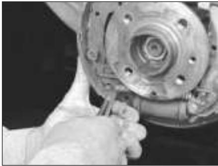
6.4a Unhook the lower return spring from the front shoe . . .
