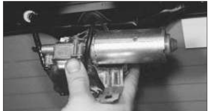
16.11a Removing the tailgate wiper motor (3-Series)
