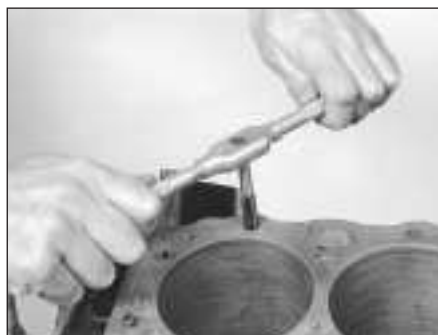
15.8 All bolt holes in the block - particularly the main bearing cap and head bolt holes - should be cleaned and restored with a tap (be sure to remove debris from the holes after this is done)
