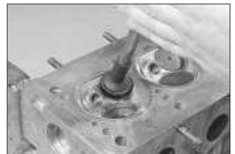
10.5 Grinding-in a valve - do not grind-in the valves any more than absolutely necessary, or their seats will be prematurely sunk into the cylinder head
