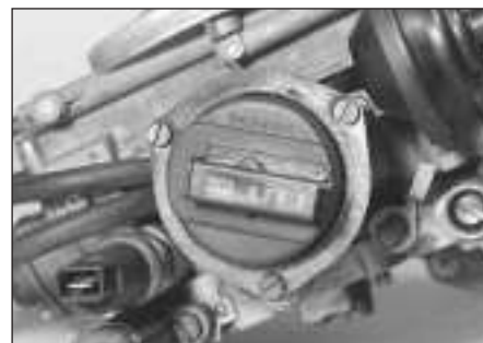
12.17 Remove the three screws and withdraw the metal ring
