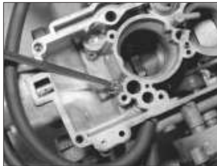
12.13a Unscrew the bypass jet from the secondary float chamber
