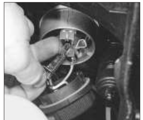
12.11 Removing the headlight bulb (do not touch the surface of the bulb with your fingers)
