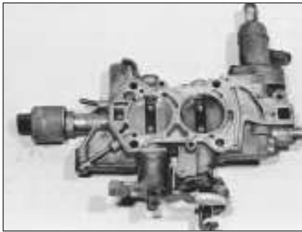
12.11a Throttle housing removed from the carburettor
