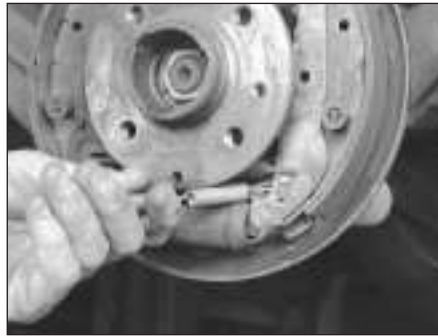
6.4b . . . then unhook it from the rear shoe and remove it
