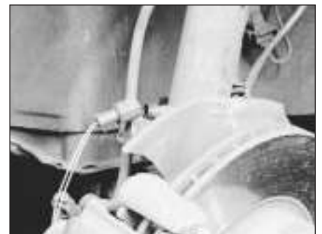
3.5f On 5-Series models, unplug the electrical connector for the brake pad wear sensor
