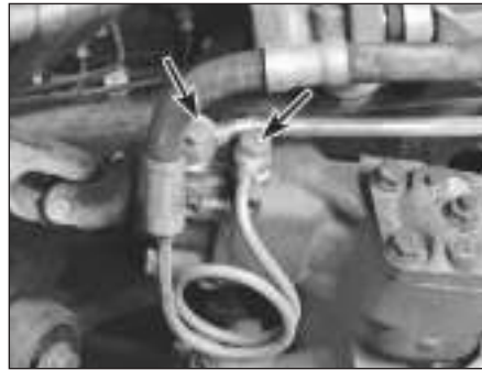
21.9 Disconnect the power steering pressure line fitting (right arrow) and the return line fitting (left arrow). Note that the return line fitting banjo bolt is larger than the bolt for the pressure line fitting (left-hand-drive shown)
