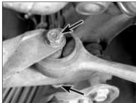
4.6b If you're removing the thrust arm, remove the nut and bolt (arrowed) that secure the rear end of the arm
