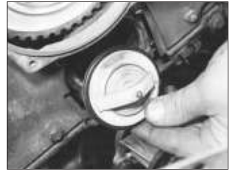
3.20b Removing the thermostat (M40 engine)
