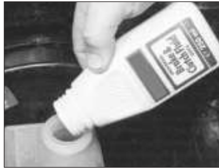
4.16 The brake fluid level should be kept above the MIN mark on the translucent reservoir - unscrew the cap to add fluid
