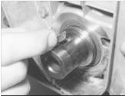
14.12 Removing the key from the groove in the nose of the crankshaft (M40 engine)
