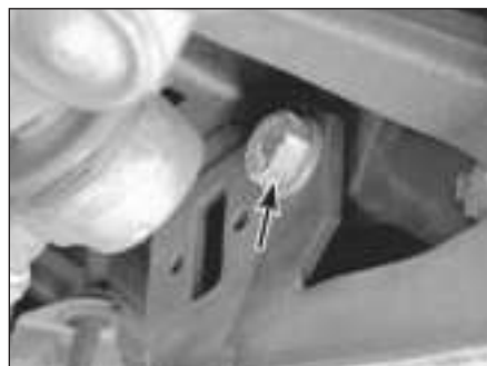
21.10b This bolt (arrowed) attaches the steering box to the body (the nut, not visible in this photo, is on the front side of the steering box)
