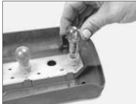
15.4b . . . then remove the bulb from the housing
