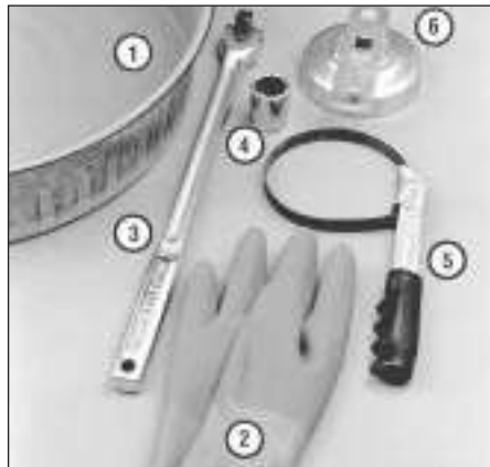
6.1 These tools are required when changing the engine oil and filter
