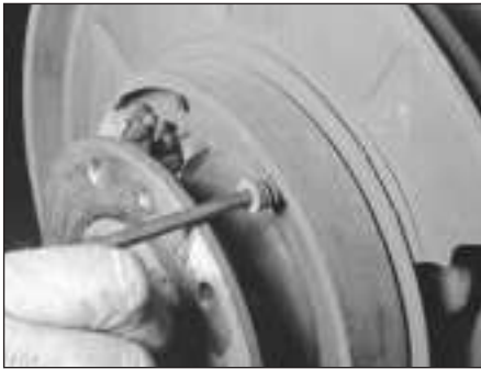
12.7c Remove the shoe hold-down springs
