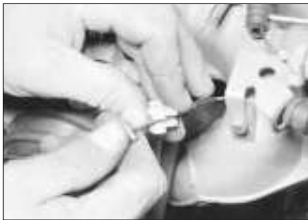
9.10b After the cable is off the throttle valve assembly, remove the plastic retainer from the cable
