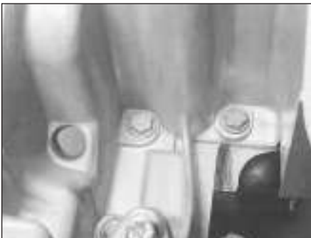
13.7a Main sump retaining bolts accessed after removal of the lower sump section on the M40 engine (engine on bench for clarity)
