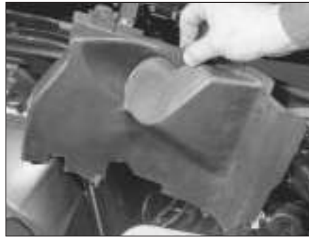
12.8 Removing the headlight rear outer cover (3-Series shown)
