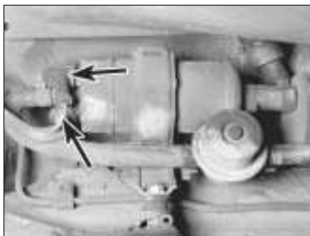
4.9 Lift up the rubber boots (arrowed) and detach the electrical connectors from the fuel pump
