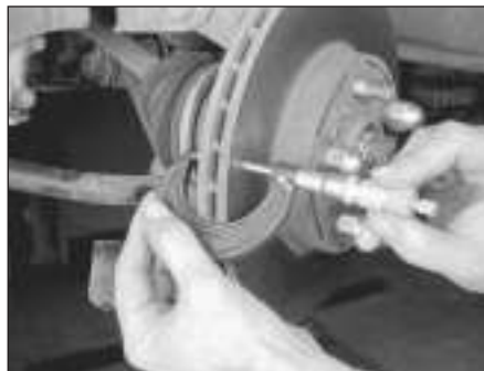
5.5 The disc thickness can be checked with a micrometer
