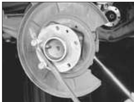
15.14c Hold the stub axle flange with a large lever while tightening the nut
