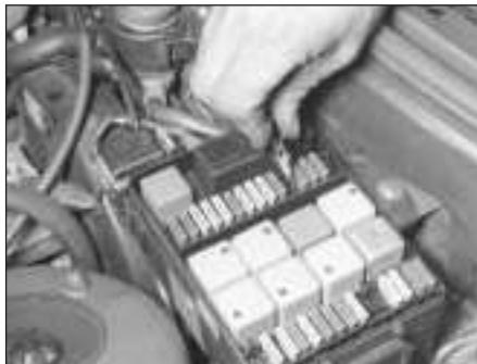
2.1a Removing the fuel pump fuse on 3-Series models
