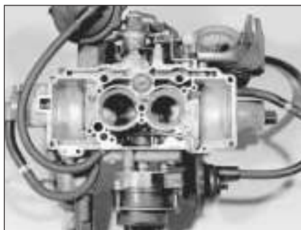
12.6c View of the carburettor main body with the cover removed
