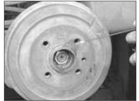
6.2b If the drum is stuck to the hub, apply penetrating oil around the hub/drum area, and give it a few minutes to loosen up any rust
