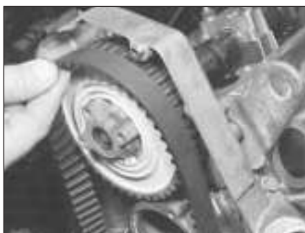
10.9b Removing the timing belt from the camshaft sprocket on the M40 engine
