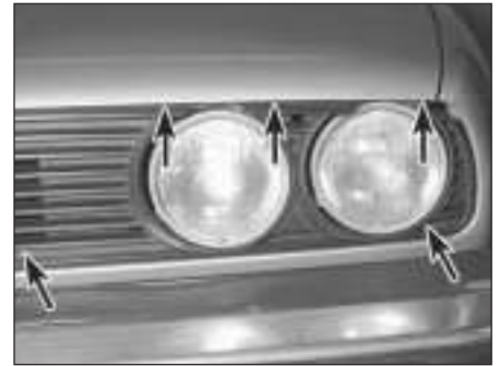
9.2b Side grille screw locations (arrowed)
