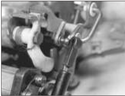
12.8 Disconnecting the vacuum unit pullrod
