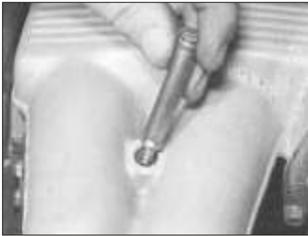
5.9a On the M40 engine, remove the nuts and special bolts . . .
