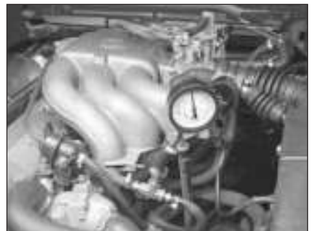
3.11 . . . and connect the gauge between the fuel feed line and the fuel rail using a tee-piece fitting
