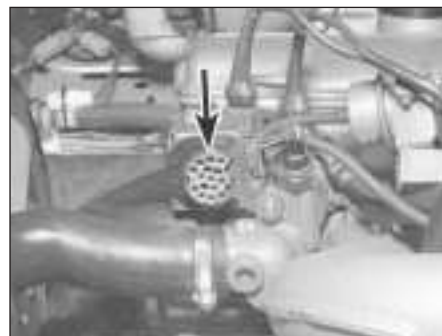
34.2a The earlier 15-pin connector (arrowed) is mounted near the front of the engine. The 20-pin connector used on later models is located in the left rear corner of the engine compartment
