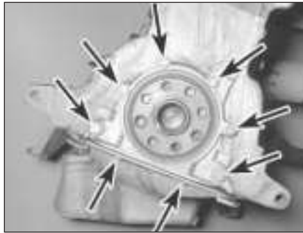
16.2 Remove the six bolts from the rear of the block and the two from underneath at the sump
