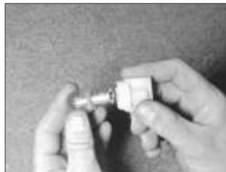
15.3c . . . then pull the bulb from the holder
