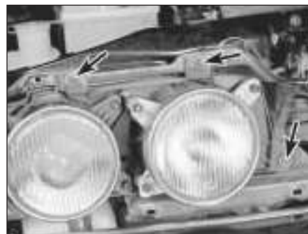
14.4 Remove the screws (arrowed) and detach the headlight housing
