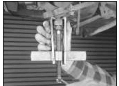
17.7 Using a puller to separate the track rod end from the steering arm
