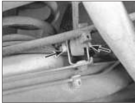
12.3a A nut and bolt (arrowed) connect each rear anti-roll bar link to the rear trailing arms (3-Series)
