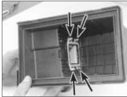
16.11b Remove the nuts (arrowed) from the air cleaner housing, and detach the airflow meter
