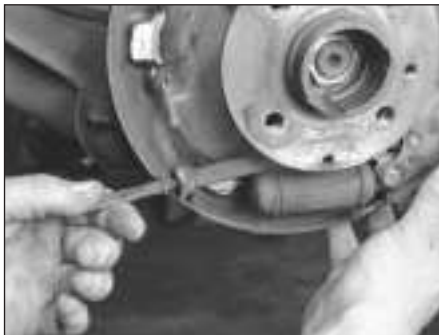
6.8 Remove the automatic adjuster assembly
