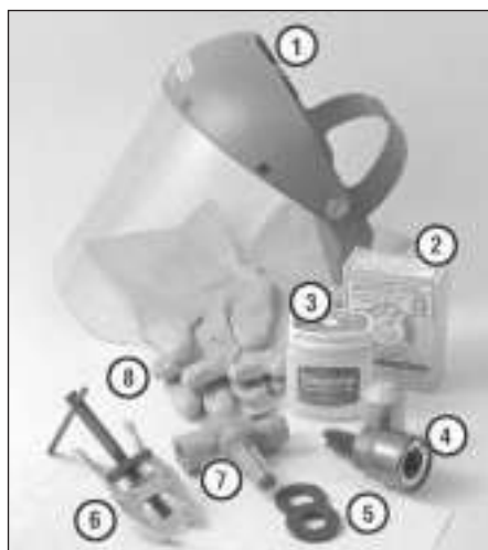
13.1 Tools and materials required for battery maintenance
