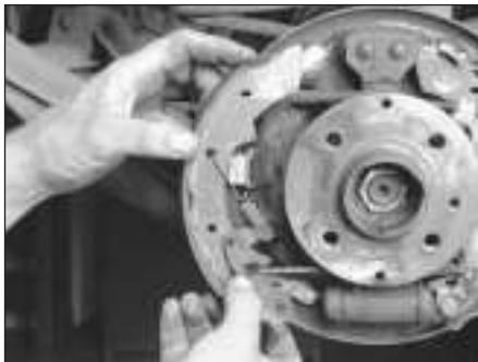
6.7 Remove the front shoe, automatic adjuster lever and spring as an assembly, then remove the lever and spring, and set them aside for attachment to the new shoe
