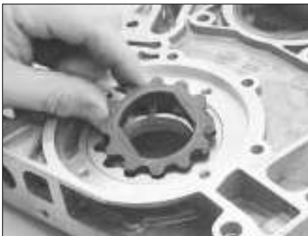
14.22a Removing the inner rotor . . .
