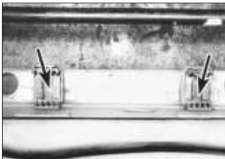
4.12 When the radiator is out, the radiator mountings can be inspected - check for signs of deterioration, and renew them, if needed
