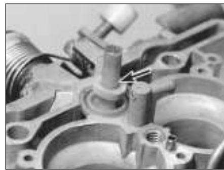
12.15c Accelerator pump seal (arrowed)
