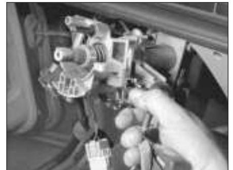
6.9 Cruise control switch removal
