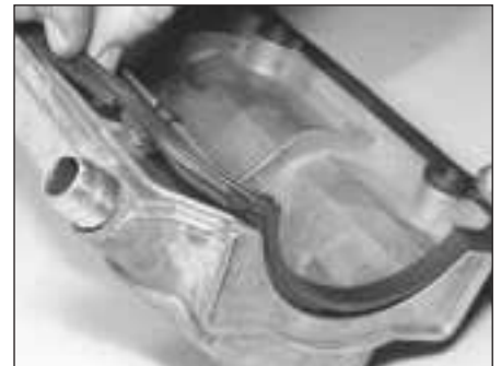
4.7c Removing the valve cover gasket on the M40 engine
