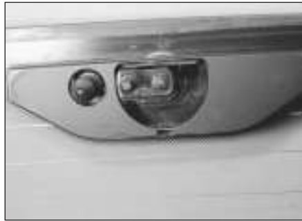
16.11c Wiper blade and pivot mechanism on the rear window (5-Series)
