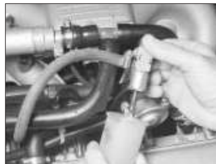
19.2 Watch for a steady, conical-shaped spray of fuel when the starter motor is operated
