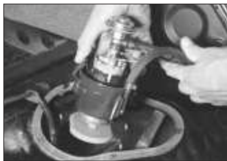
4.18d . . . then pull the fuel pump straight up and out of the turret at the bottom of the fuel tank (keep all the fuel lines intact)
