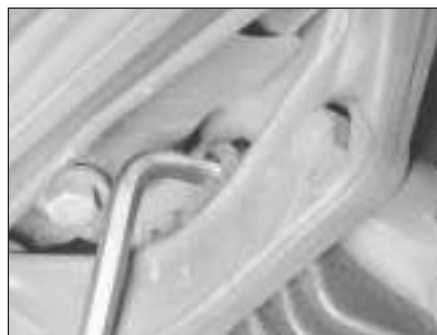
17.2 Remove the differential filler/level plug with an Allen key, and make sure the lubricant is level with the bottom of the hole
