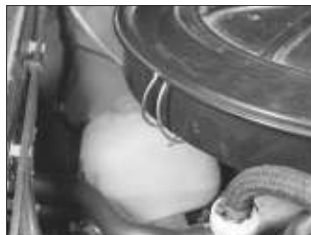
8.2a Release the air cleaner cover spring clips . . .
