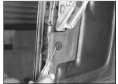
10.8b . . . prise the retainer out
