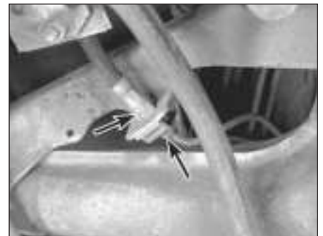
14.3 Disconnect the brake hose (left arrow) from the fitting on the metal brake line (right arrow) at this bracket
