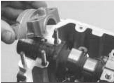
8.17a Removing the camshaft bearing caps . . .
