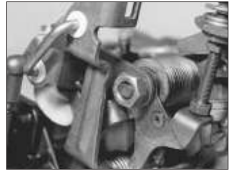
12.10 Primary throttle lever securing nut - if removed, take care not to disturb the return spring
