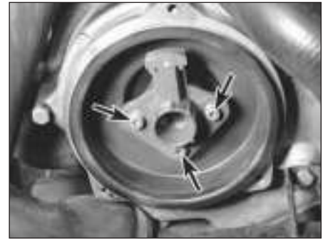
8.19 Remove the rotor screws (arrowed) with an Allen key, and pull the rotor off the shaft
