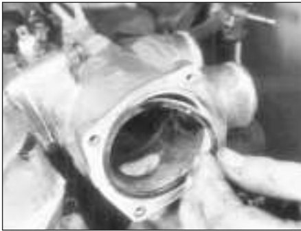
3.15 On M20 and M30 engine models, after the housing and thermostat have been removed, take the O-ring out of the housing and clean the recess in the housing to be sure of a good seal upon reassembly
