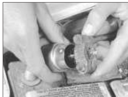
13.8d When cleaning the cable clamps, all corrosion must be removed (the inside of the clamp is tapered to match the taper on the post, so don't remove too much material)
