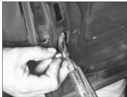
10.10 Support the bonnet and withdraw the pin
