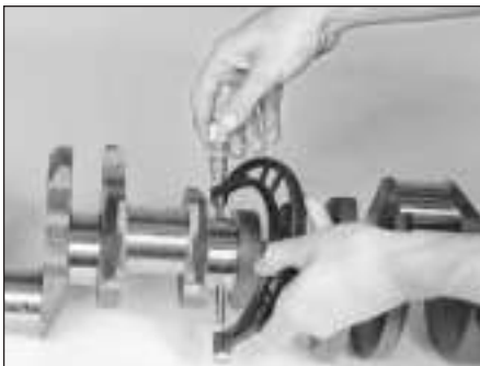
19.6 Measure the diameter of each crankshaft journal at several points to detect taper and out-of-round conditions
