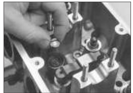
8.20b . . . and thrust discs . . .
