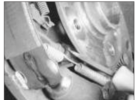
6.2c If the brake shoes have worn a groove in the drum and it won't come off, insert a thin flat-bladed screwdriver through one of the wheel bolt holes in the flange, and loosen the automatic adjuster mechanism (for the sake of clarity, the drum has already been removed in this photo, and the screwdriver is being inserted underneath the flange instead of through a wheel bolt hole)
