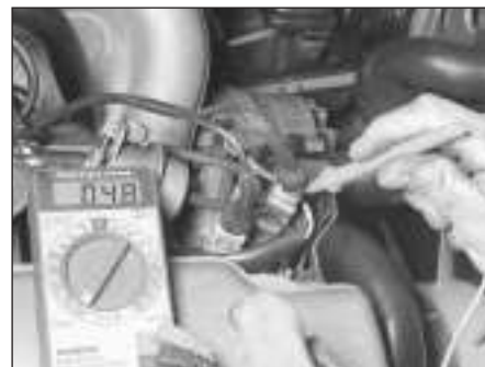
19.4 Check for a voltage signal on the black/yellow wire of the thermotime switch when the ignition is on
