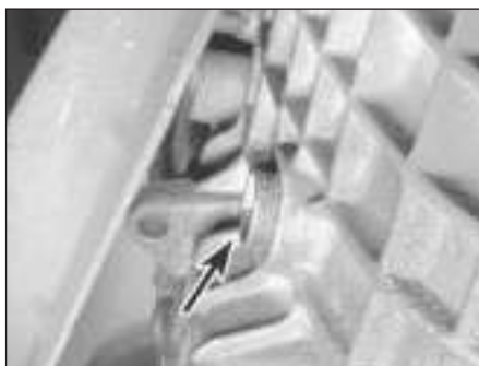
16.2 Use a large Allen key to remove the filler/level plug (arrowed) and check the lubricant level with your little finger. It should be level with the bottom of the hole - if it's low, add lubricant
