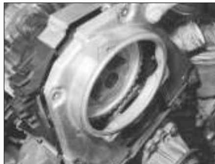
9.9b Removing the upper timing belt cover on the M40 engine
