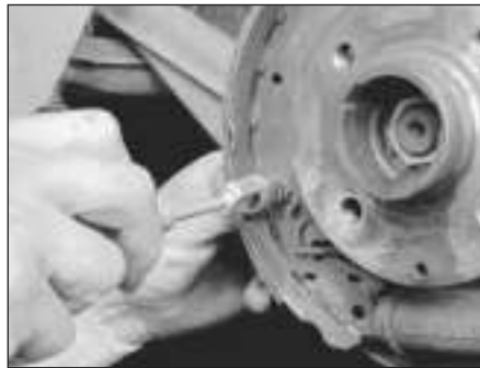
6.6a Remove the front shoe hold-down spring . . .
