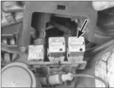
3.5 As a safety precaution, before performing a compression check, remove the cover and the main relay (arrowed) from the left side of the engine compartment to disable the fuel and ignition systems (525i model shown, other models similar)
