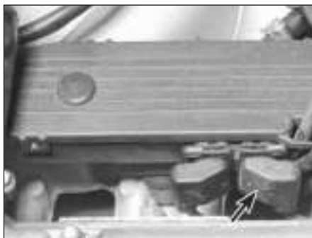
12.7b On later 5-Series models, the pulse sensor connector (arrowed) is located next to the valve cover
