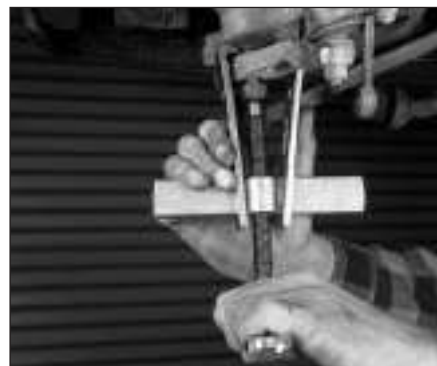
4.7b You can separate the thrust arm balljoint from the steering arm with a puller . . .
