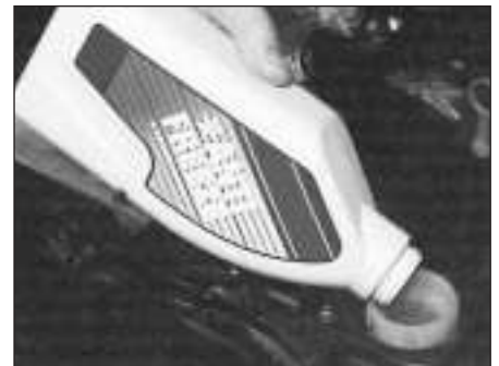
4.9d Adding antifreeze mixture
