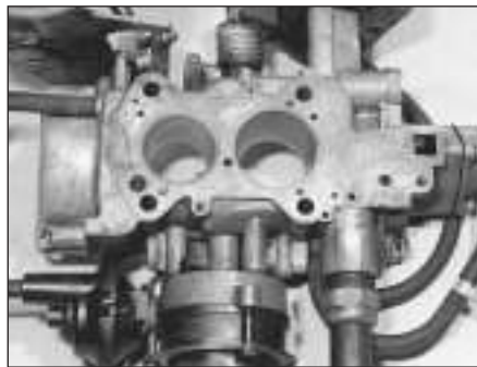
12.11b Underside of the main body with throttle housing removed - note gasket
