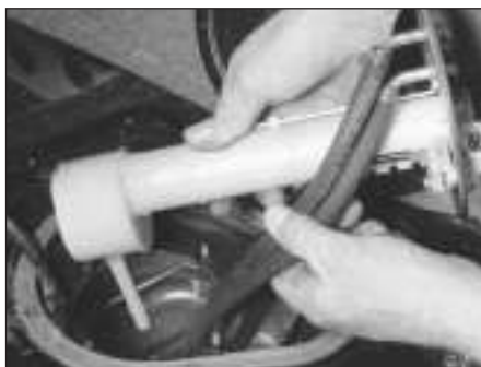
4.18c On later Motronic systems, first remove the fuel level sender unit . . .
