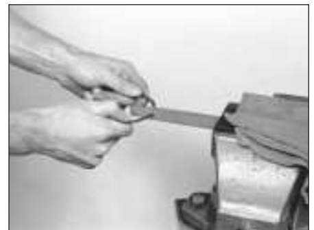
22.5 If the end gap is too small, clamp a file in a vice, and file the ring ends (from the outside in only) to enlarge the gap slightly
