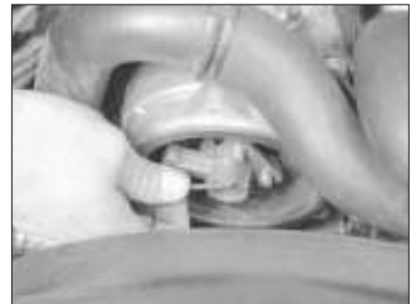
15.11b Use an Allen key to remove the screws, then lift the rotor off the shaft (later models)
