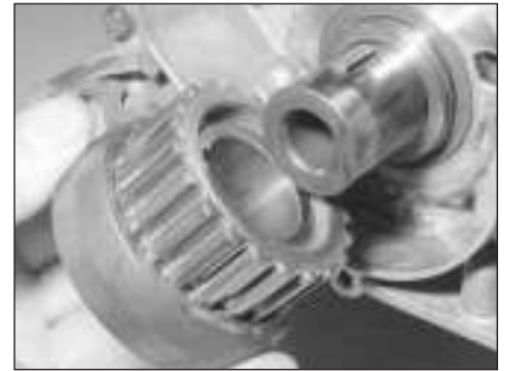
10.12c Removing the crankshaft sprocket from the front of the crankshaft
