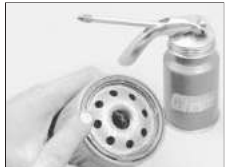
6.16 Lubricate the oil filter sealing ring with clean engine oil before refitting the filter on the engine
