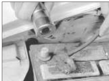
13.8c Regardless of the type of tool used on the battery posts, a clean, shiny surface should be the result
