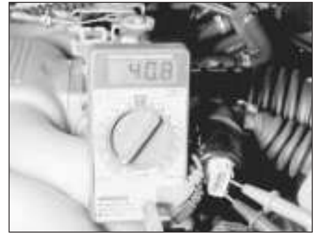
21.21 Check the idle air stabiliser valve resistance on the two outer terminals on later Motronic systems - it should be about 40 ohms
