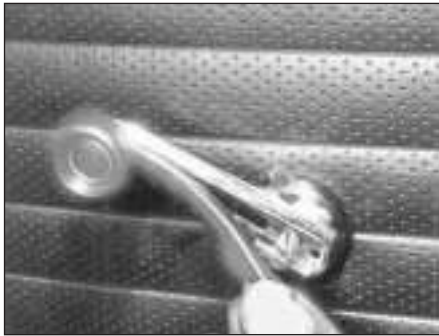
12.3 On models without electric windows, prise off the window regulator handle trim piece for access to the retaining screw
