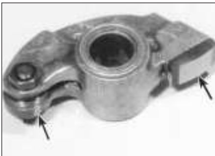
9.18 Look for signs of pitting, discoloration or excessive wear on the ends of the rocker arms where they contact the camshaft and the valve stem tip
