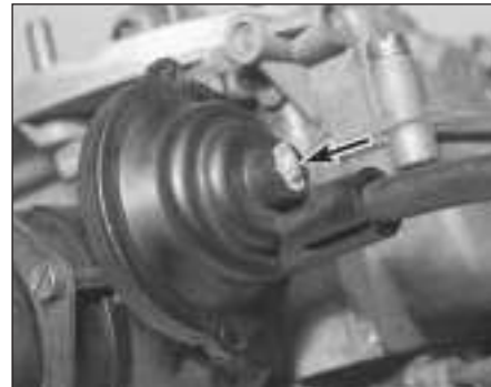
12.20 If adjustment is necessary, turn the screw (arrowed) on the end of the pulldown unit
