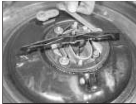
8.6a Unscrew the four air cleaner-to-carburettor nuts . . .
