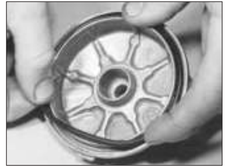
6.19 Renewing the rubber O-ring in the cover
