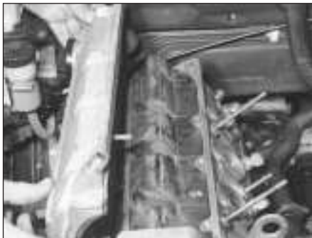
4.7a Removing the valve cover on the M40 engine
