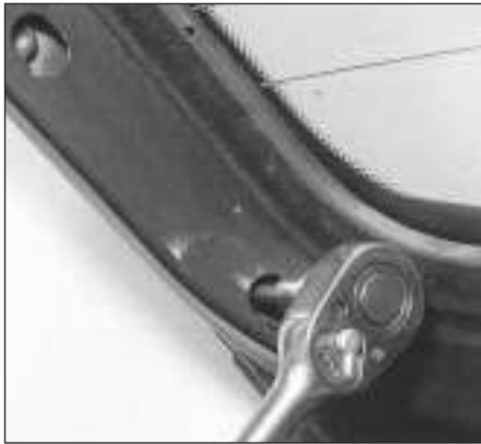
14.14 Unscrewing the hinge mounting bolts (5-Series)
