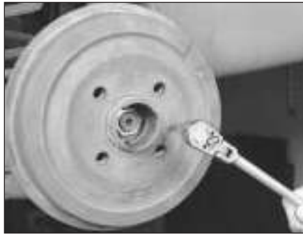
6.2a Removing the drum retaining screw
