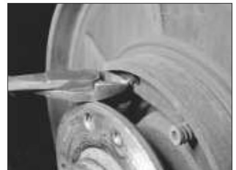
12.7b Remove the upper shoe return spring
