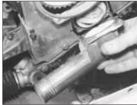
3.20a Removing the elbow from the cylinder head (M40 engine)
