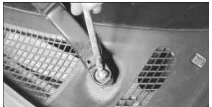
16.2b After removing the nut, use a magnet to lift out the metal washer
