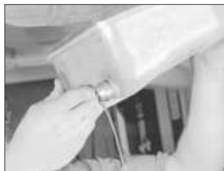
28.7 Lower the sump from the transmission
