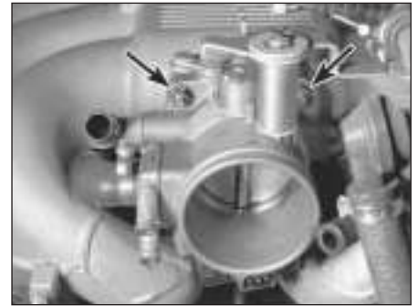
17.11 Remove the nuts (arrowed) and lift the throttle body from the intake manifold (the two lower bolts are hidden from view)
