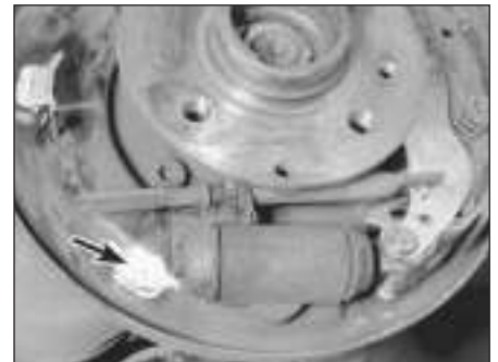
6.11 Before you fit the new shoes, apply some high-temperature brake grease to the friction surfaces where the inner edge of the shoe slides on the brake backing plate - when you refit the automatic adjuster mechanism, make sure each end engages properly with its respective notch in the brake shoe
