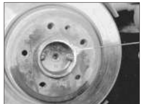
5.6c If the disc is stuck to the hub, spray some penetrating oil onto the area between the hub and the disc, and give the oil a few minutes to separate the two parts
