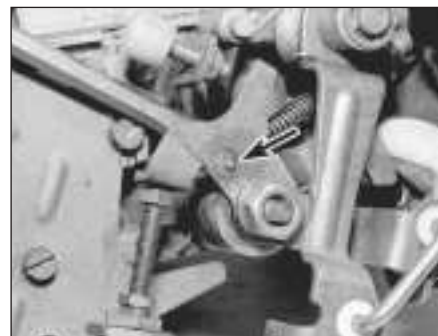
12.3 Using a screwdriver to disconnect the accelerator pump linkage (arrowed)
