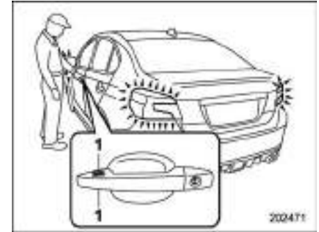
1) Door lock sensor (above and below)
