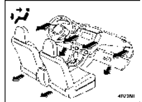
Bi-level: Instrument panel outlets and foot outlets
