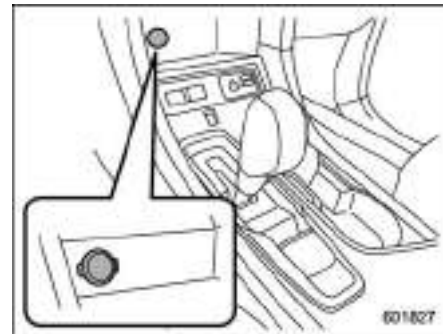
Power outlet below the climate control dials
