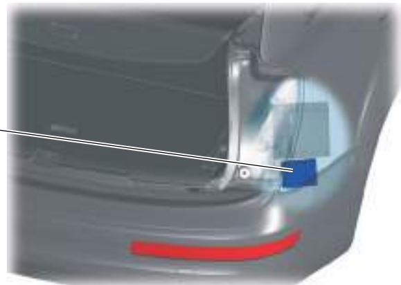
Installation location of the aerial reader unit for entry authorisation for keyless entry system J723
