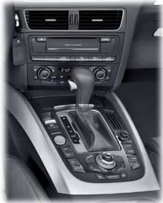
EV mode switch and shift control with tip-S function
