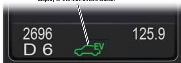
Display of activated EV mode in the display of the instrument cluster
