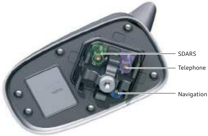
Roof aerial R216 (North America)
