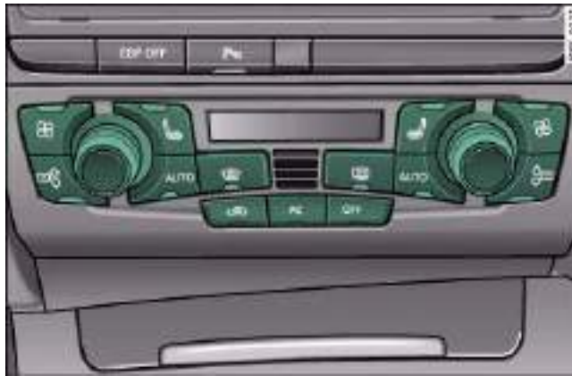
Fig. 116 Air conditioner controls
