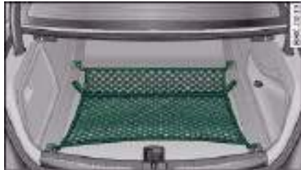
Fig. 84 Stretch net laid out
