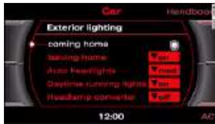
Fig. 52 MMI display: Exterior lighting
