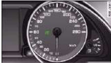
Fig. 139 Indicator lamp for the cruise control system - lights up when the system is operating.
