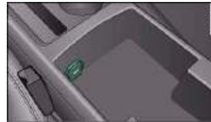
Fig. 102 Electrical socket in the centre console
