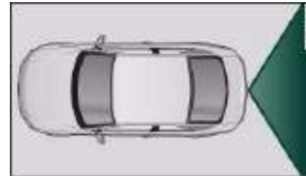
Fig. 158 Viewed from above: Area covered by the reversing camera
