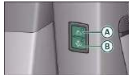
Fig. 40 Front end of the driver's door: Switches for interior monitor and tow-away protection
