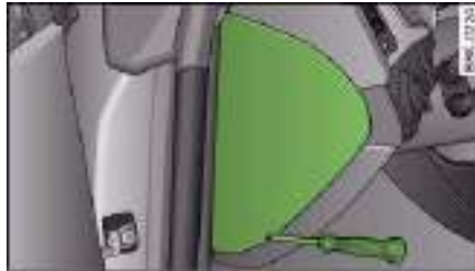
Fig. 253 Left side of dash panel: Fuse cover
