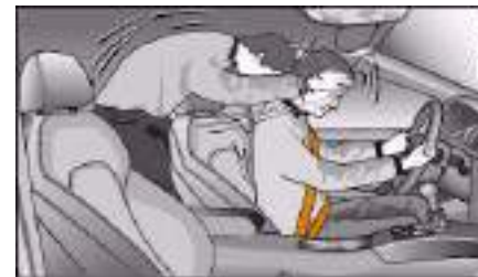
Fig. 181 A rear passenger not wearing a seat belt can be thrown forwards
