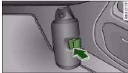
Fig. 236 Fire extinguisher in footwell on front passenger's side
