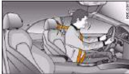
Fig. 177 Driver protected by the properly worn seat belt during a sudden brake manoeuvre
