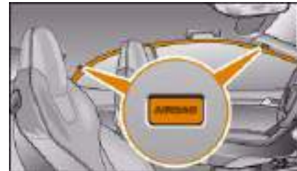
Fig. 193 Location of head-protection airbags above the doors
