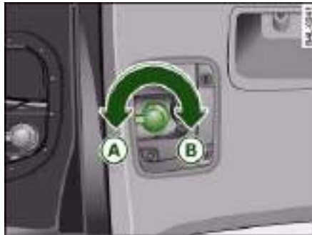
Fig. 257 Diagram: Bulb holder with a bayonet fastener
