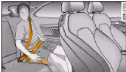
Fig. 200 A category 2/3 forward-facing child seat (without backrest) fitted on the rear seat
