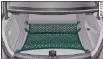
Fig. 84 Stretch net laid out
