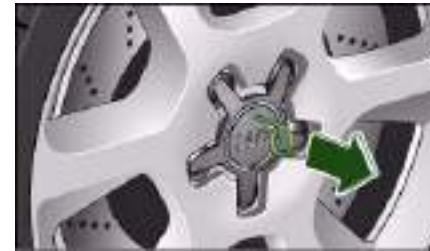
Fig. 271 Changing a wheel: Removing a hub cap
