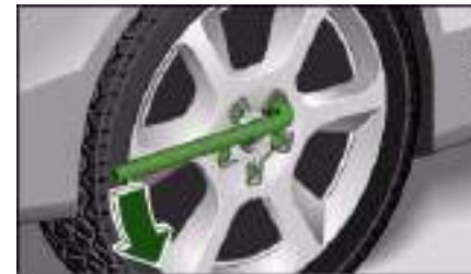
Fig. 272 Changing a wheel: Loosening wheel bolts
