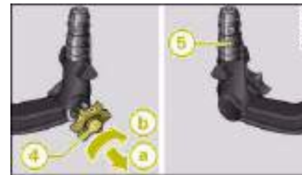
Fig. 239 Removable towing bracket: Setting the spring mechanism to the "ready" position
