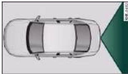
Fig. 189 Viewed from above: Area covered by the reversing camera
