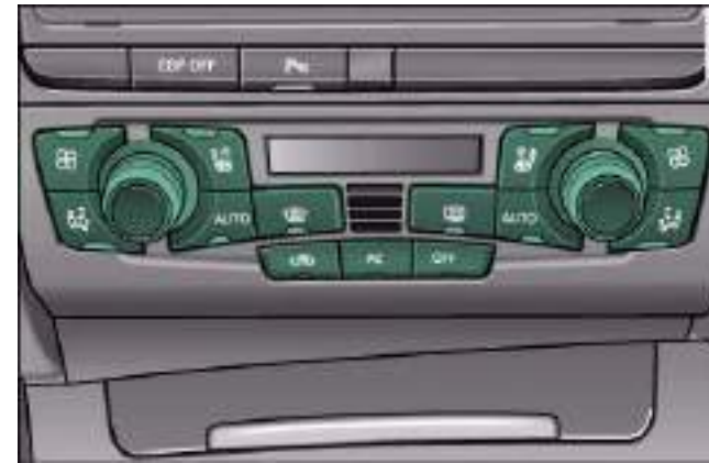
Fig. 112 Air conditioner controls
