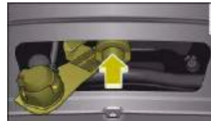
Fig. 240 Removable towing bracket: Inserting the ball joint
