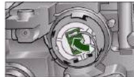
Fig. 297 Inserting bulb for dipped headlights
