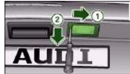
Fig. 310 Boot lid: Removing number plate light
