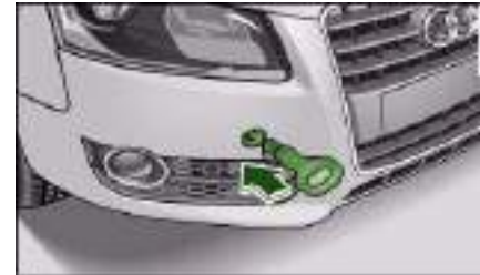
Fig. 281 Front bumper: Fitting the towing eye
