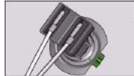
Fig. 296 Bulb with connector: The lug on the base of the bulb is highlighted
