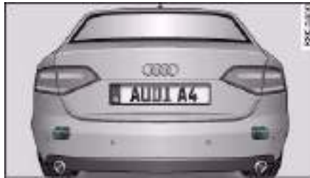
Fig. 163 Rear bumper: Position of radar sensors (not externally visible)
