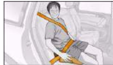
Fig. 229 A category 2/3 forward-facing child seat (without backrest) fitted on the rear seat
