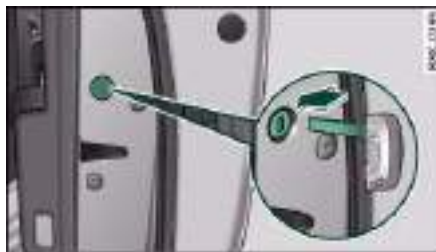
Fig. 44 Door: Locking the door manually
