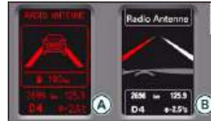
Fig. 160 Instrument cluster: lane assist switched on and in warning mode
