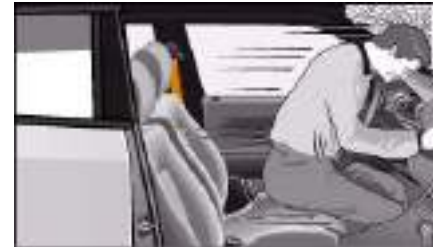
Fig. 206 A driver not wearing a seat belt can be thrown forwards
