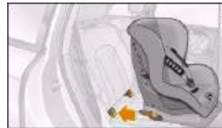
Fig. 231 The ISOFIX child safety seat is pushed into the protective sleeves.
