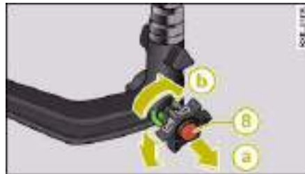
Fig. 243 Removable towing bracket: Removing the ball joint
