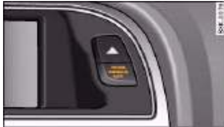
Fig. 223 Lamp indicates that front passenger's airbag has been deactivated via key-operated switch
