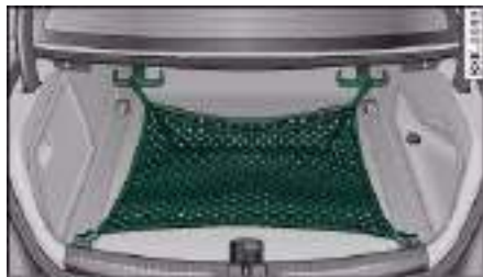
Fig. 85 Stretch net attached in position as retaining net
