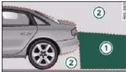
Fig. 190 Side view: ①: Area covered by the reversing camera; ②: area NOT covered by the reversing camera
