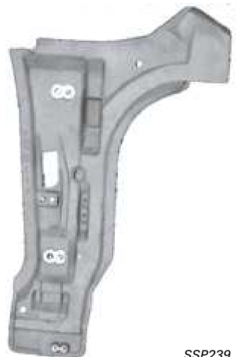
A-pillar large cast parts (A2)
