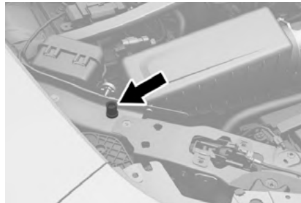
Remote Negative (-) Post Location
