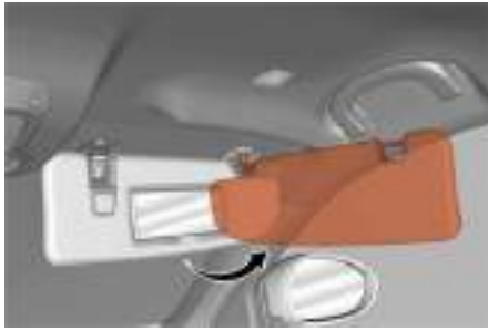
Rotate Sun Visor Toward Passenger Window
