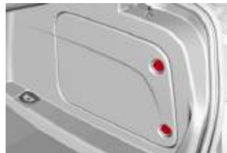
Battery Access Panel
