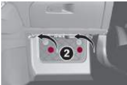
Release Hooks On Footboard
