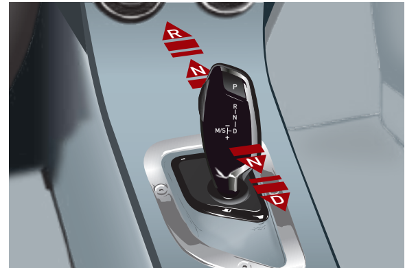
Engaging Selector Lever positions D, N, R. (LHD Selector shown)
