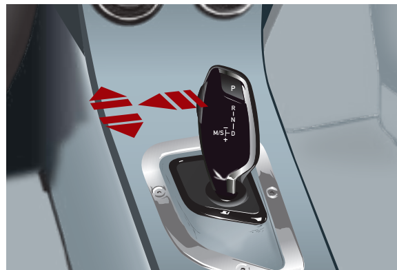
Activating Manual Operation. (LHD Selector shown)
