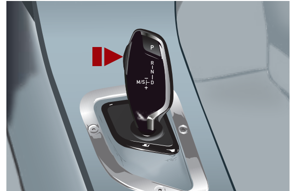
Selector Lever Lock. Press button. (LHD Selector shown)
