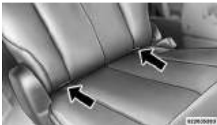
ISOFIX Anchorages (Second Row Anchorages Shown)
