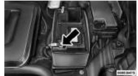
Positive Battery Post
