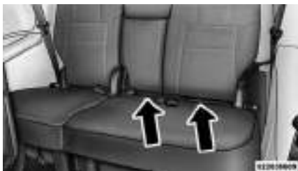
ISOFIX Anchorages (Third Row 60/40 Anchorages Shown)
