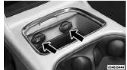
Super Console Outlets
