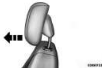
Active Head Restraint (Tilted)
