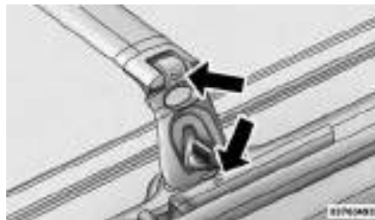
Crossbar To Side Rail Installation
