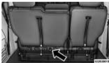
ISOFIX Anchorages (Third Row 60/40 Anchorage Shown)
