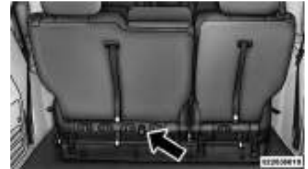
ISOFIX Anchorages (Third Row 60/40 Anchorage Shown)
