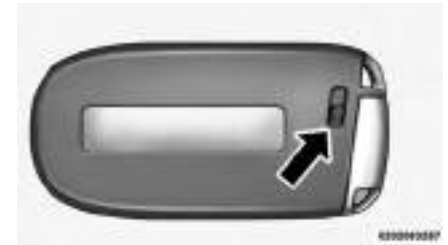
Mechanical Latch On The Back Of The Key Fob
