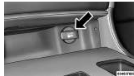
Front Power Outlet
