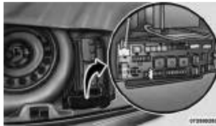
Rear Power Distribution Center
