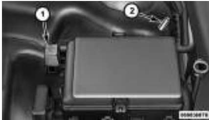
Remote Battery Post Locations
