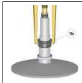
Removing the tightening ring (1b)
