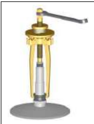
Removing the tightening ring (1b)
